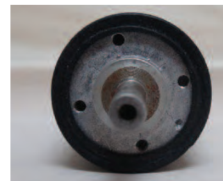
5. Hoof buffer with new bladder properly covering end of buffer.
