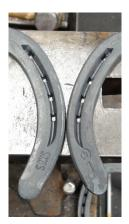
Line up the toes of the SX-8 Select (left) and the regular SX-8 (right) at the edge of the anvil to see the additional length of the SX-8 Select. Nail placement is almost identical for an extended fit without having to go up a size. The widest part of the shoe will still be where you need it.
