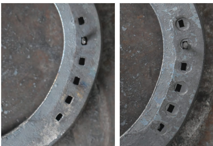
Left: New shoe. Right: Modification of new shoe to better accept a Slim blade nail. Here again, I lightly drive a stud punch into the foot side of the shoe at low heat.
