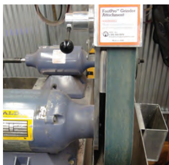
A zirconia belt with material loading present.
