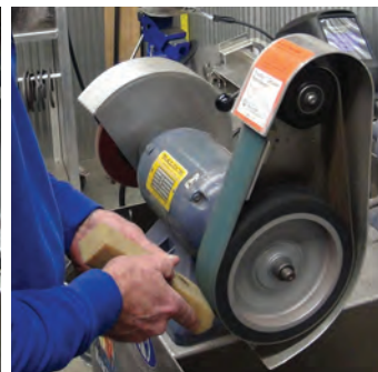
Turn on grinder. Maintain contact with belt and sweep side-to-side to clean.
