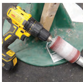
A hoof buffer sleeve loaded with hoof material.
