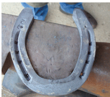
Inside heel of the shoe forged to allow the hoof to sink.
