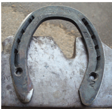
The shoe ground, drilled and tapped.
