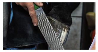
The innovative and unique manufacturing process of the Diamond Max Glide creates a high-quality rasp and file; 10% wider than the standard rasp. The rasp side features a 9-tooth pattern with slightly smaller teeth, and a file side with the chip breaker cut for a smooth finish.
