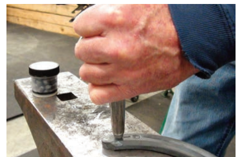
This image shows the Bloom C11 Stud Set Punch being used. Be sure to align stud in hole of punch.
