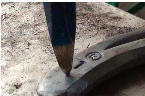
Center Punch desired location for studs before drilling.
