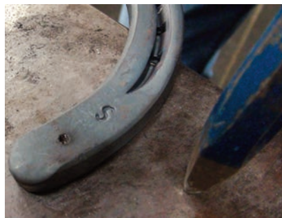
This mark will help with drilling in the desired location.
